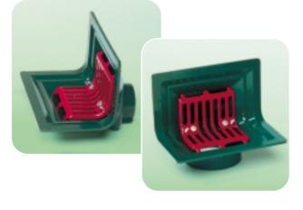
**Caroflow** Two-Way Threaded roof outlets are designed for use at the intersection of horizontal and vertical surfaces, i.e. a balcony and parapet wall, and can be used to drain off vertically or horizontally. Available in either LM6 Aluminium Silicon casting alloy to BS1490:1970 for most roof finishes or in leaded gunmetal to BS1400:1985 for use with lead or copper-clad roofs or for connection to copper pipework. They are female parallel threaded to BS21:1985.
